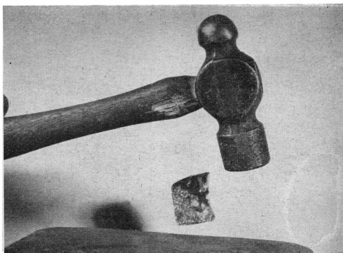
PURE: Properly molten, titanium bounces under hammer blow. High price—$5 a pound—is due to difficulty of refining.
